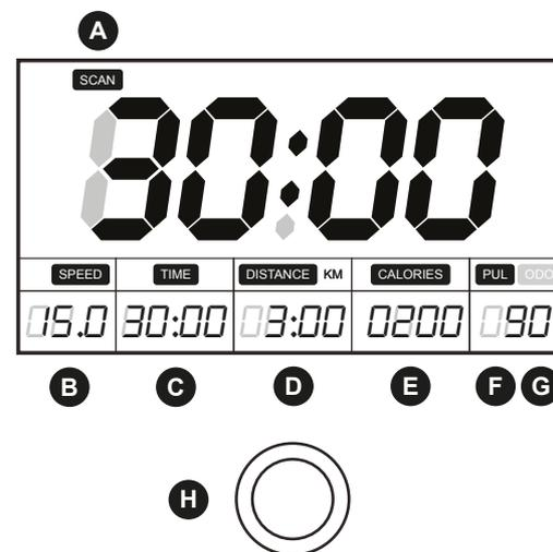
To select a function, press the selection button (**H**) until the desired function is displayed.
